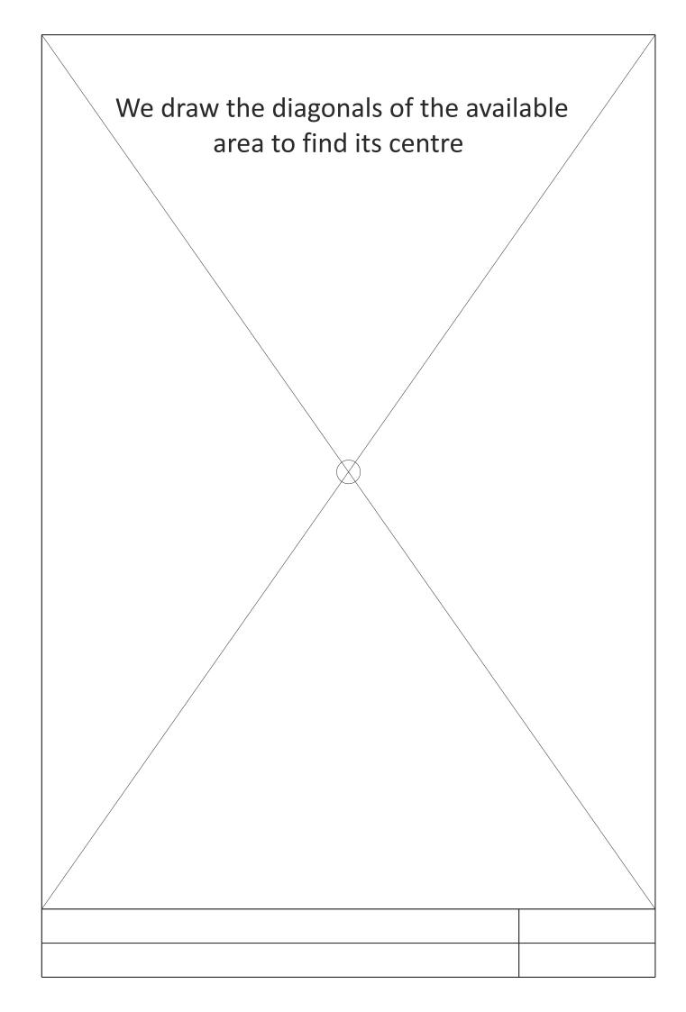
Now, we keep only a small X on the centre, and we draw a vertical line through it. This will be the simmetry axis, and has to be perpendicular to the horizontal lines of the margin. Therefore, we will have to use our set squares to do so. NOT PRINT THIS PAGE NOT PRINT THIS PAGE NOT PRINT THIS PAGE NOT PRINT THIS PAGE DO NOT PRINT NOT PRINT THIS NOT PRINT THIS PAGE NOT PRINT THIS
